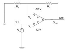
a) **Practical work**: Adjust  $V_I(t) = 8 \operatorname{Sin}(2\pi ft)$  Volt where f = 500 Hz. Connect CHI and CHII of the oscilloscope as in the figure. Use **Display menu** of the oscilloscope change **format** to XY. Draw the obtained Hysteresis curve. This curve shows  $V_I$  (CHI in x axis) versus  $V_{out}$  (CHII in y axis) characteristics of the bistable circuit.
