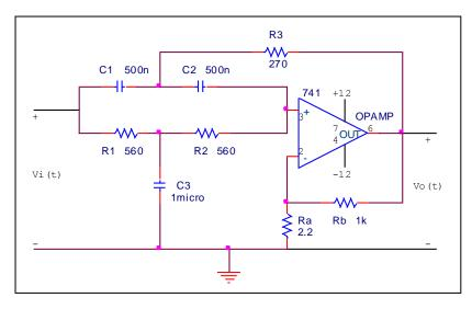
Sketch the magnitude and the phase of the response function H(j)=Vo(jw)/Vi(jw). Indicate half-power angular frequency values  $w_{c_1}$ ,  $w_{c_2}$ , the angular frequency  $w_o$  where minimum of response is attained, and the stop-band bandwidth,  $\Delta w$ .
