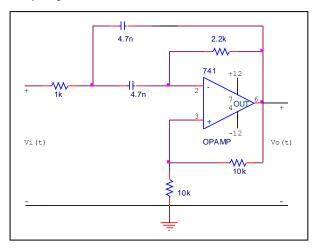
Determine and sketch the magnitude and the phase of the response function H(jw)=Vo(jw)/V(jw). Indicate the half-power angular frequencies  $w_{c_1}$ ,  $w_{c_2}$ , and center frequency  $w_{o_1}$  and bandwidth,  $\Delta w$ .
