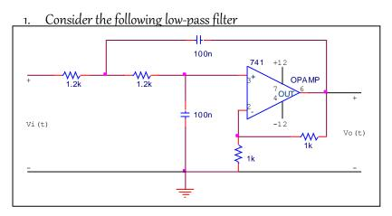
Determine and sketch the magnitude and the phase of the response function H(jw)=Vo(jw)/V(jw). Indicate the half-power frequency  $w_c$ .
