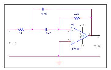
Sketch the magnitude and the phase of the response function H(j)=Vo(jw)/Vi(jw). Indicate half-power angular frequency values  $w_{c1}$ ,  $w_{c2}$ , the angular frequency  $w_0$ , and the pass-band bandwidth,  $\Delta w$ .
